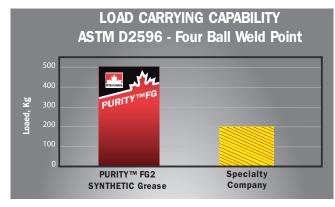
PURITY FG2 Synthetic grease provides higher load carrying capability than a specialty lubricant suppliers' synthetic food grade grease, so it's ideal for food processing applications running under heavier loads.
