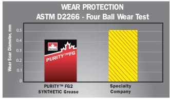
PURITY FG2 Synthetic delivers equal wear protection to a specialty lubricant suppliers' synthetic food grade grease. Less wear means fewer production upsets, higher productivity and lower maintenance costs.
