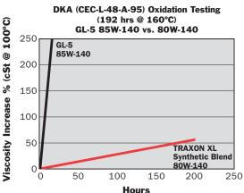
In the DKA oxidation test, product performance is measured by how much harmful viscosity increase will occur over time (therefore, the flatter the line the better). TRAXON XL Synthetic Blend clearly outperforms the GL-5 85W-140 gear oil.
