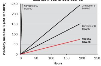
In the DKA oxidation test, product performance is measured by how much harmful viscosity increase will occur over time (therefore, the flatter the line the better). Compared to these competitors, Petro-Canada's TRAXON 80W-90 with its advanced formulation is clearly superior.
