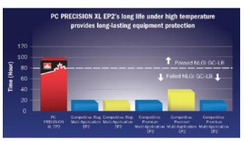
ASTM D3527 Bearing Life Performance Test at 160°C (320°F), 1000 rpm speed and 111 N thrust load
