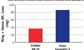
HYDREX provides up to 2x better wear protection than a global competitor.
