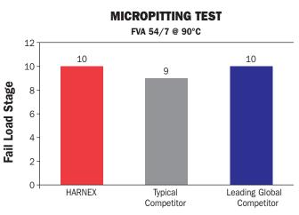
HARNEX resists micropitting by dramatically reducing scuffing wear in gears. It meets the FVA 54/7 Micropitting Test (Fail 10) required by most European gearbox manufacturers.
