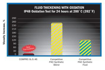
New and Improved COMPRO XL-S shows strong resistance to oil thickening, which can improve compressor efficiency and lower energy consumption.
