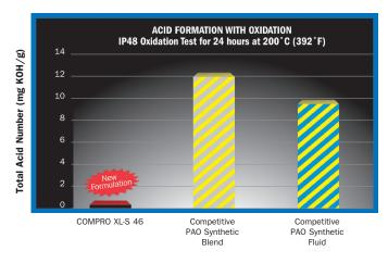
Tests show COMPRO XL-S can control build-up of acidic by-products due to oil oxidation.
